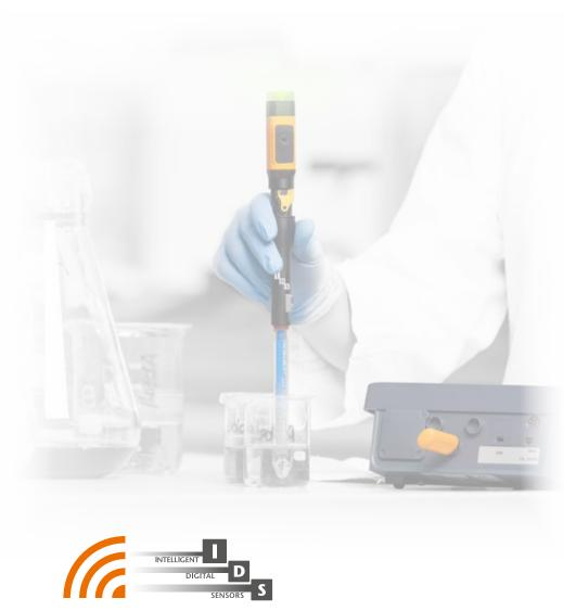
The IDS wireless sensors must be calibrated with any IDS bench or portable meter for storing the calibration data in the sensor head.
